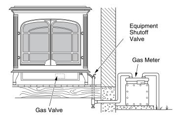
Figure 44 - Checking Gas Joints for Natural Gas Burner System (Oxford™ Model Shown)
